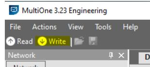
A window will open allowing you to set which features to override on the power supply. Deselect all and leave **only the check button** on characteristics '*Dimming Interface*', and/or '*Dynadimmer*', as shown below. Then press the “*Write*” button to overwrite the new configuration on the power supply of the luminaire.
