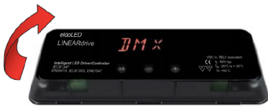
A Removing the cover
