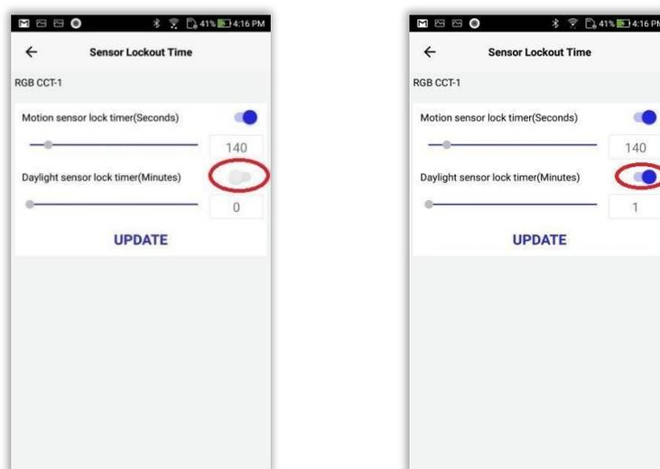
Figure 33 Min value 1 on enabling the property
