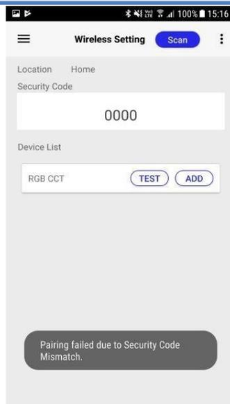
Figure 15 Alert on security code mismatch
