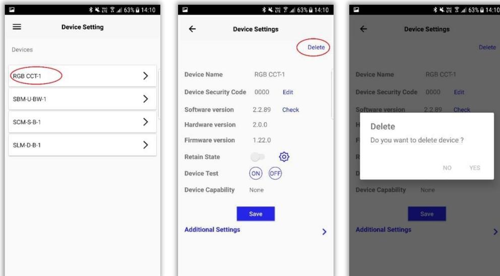
Figure 114 Deleting device
