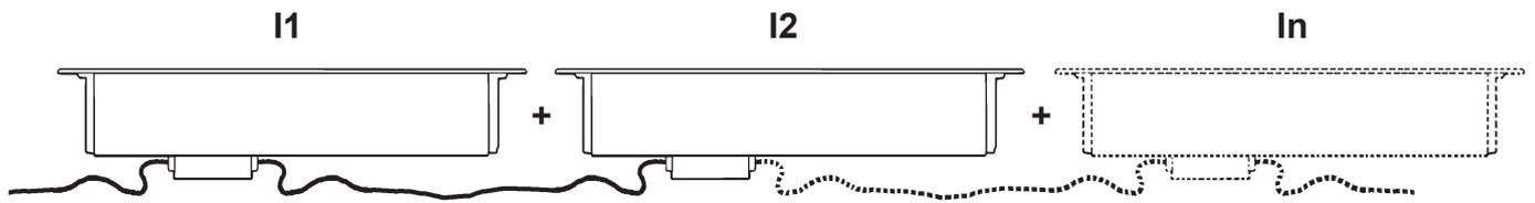
$I_{tot} = I_1 + I_2 + \dots + I_n = \max 9A$   $9A \Rightarrow$
