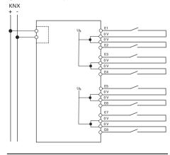
An installation with Y bell wire or J-FY flat i webbed bell wire is permitted.
